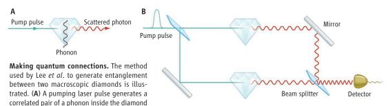
as well as a scattered photon. (B) The scattered photons from two diamonds are brought together for interference and detection. When one photon is detected, the two diamonds coherently share a phonon. Thus, the quantum state created has the hallmarks of quantum entanglement.
