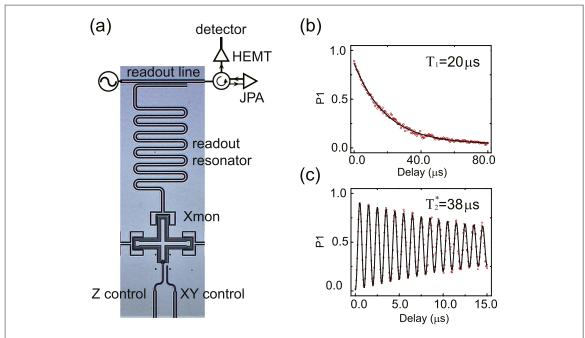
**Figure 1.** (a) An optical micrograph of a single cross-shaped Xmon qubit. (b) Energy decay of the qubit, giving a relaxation time of  $T_1 = 20 \ \mu s$ . (c) Ramsey fringes of the qubit, giving a pure decoherence time of  $T_2^* = 38 \ \mu s$ .
