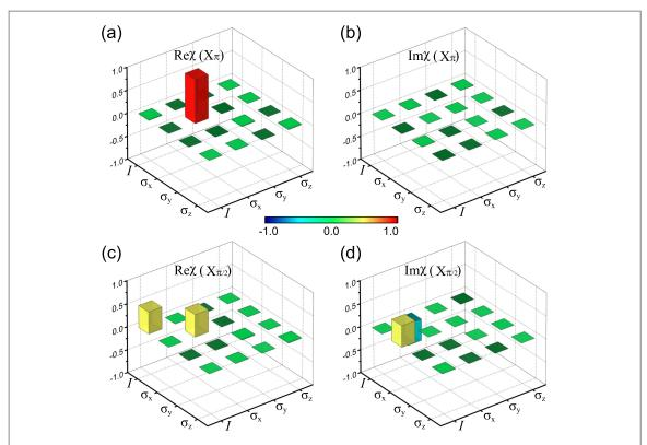
**Figure 3.** The experimental measurement of  $\chi$  matrices for (a), (b)  $X_{\pi}$  and (c), (d)  $X_{\pi/2}$  rotations. The left and right panels are the real and imaginary parts of the two  $\chi$  matrices, respectively.
