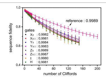
**Figure 6.** Randomized benchmarking measurement for a set of single-qubit STA quantum gates. The reference and interleaved sequence fidelities are displayed as functions of the number of Cliffords. Each sequence fidelity is averaged over k = 50 randomized operation (see text), with its standard deviation from the mean shown as an error bar. All the gate fidelities are calculated and shown in the figure.
