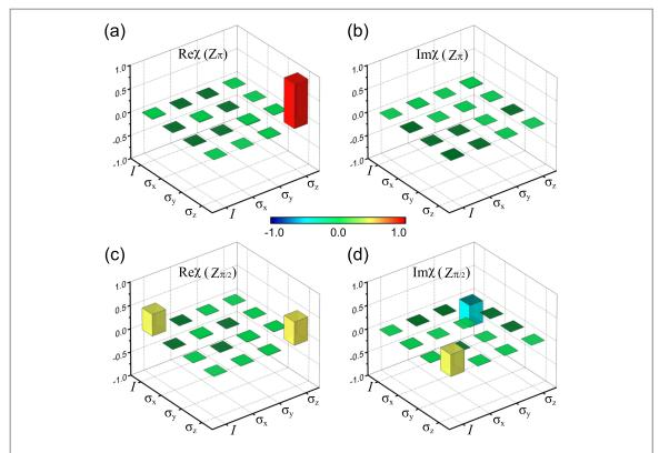
**Figure 4.** The experimental measurement of  $\chi$  matrices for (a), (b)  $Z_{\pi}$  and (c), (d)  $Z_{\pi/2}$  rotations. The left and right panels are the real and imaginary parts of the two  $\chi$  matrices, respectively.
