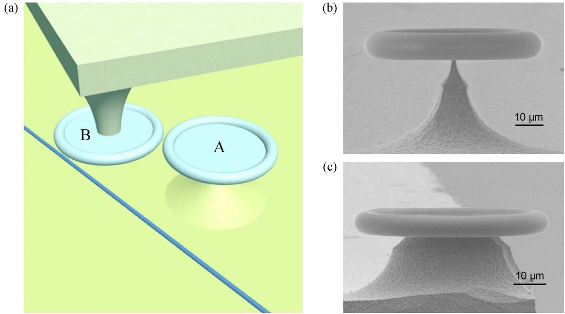
Fig.1. (a) Schematic diagram of the coupling geometry between two microtoroid resonators. (b) and (c) Scanning electron microscope images of the microtoroid with tiny silicon pillar and the microtoroid at the corner of a silicon chip, respectively.
