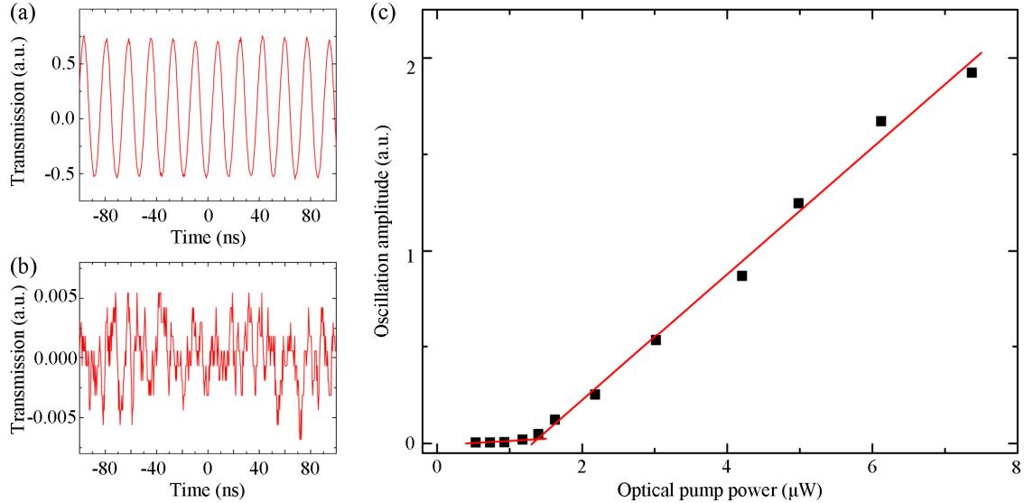
Fig. 2. (a) and (b) Optical transmitted powers above and below the threshold, respectively. (c) Measured oscillation amplitude versus optical pump power.
