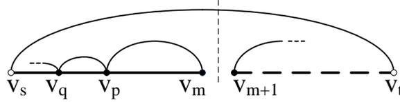
Fig. 2: The structure of  $A(s, t)$ :  $f'_1(s, m)$  is the minimum total interference created by the nodes on the solid segment from  $v_s$  to  $v_m$  (the left endpoint  $v_s$  excluded), and  $f'_2(m+1, t)$  that on the dashed segment from  $v_{m+1}$  to  $v_t$  (the right endpoint  $v_t$  excluded).
