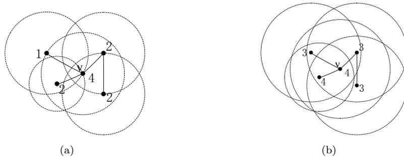
Fig. 1: The protocol interference model: straight lines are the links; the dashed circle centered at a node indicates its interference range; and the number beside a node is interference on it. (a)  $\delta = 0$ , and (b)  $\delta = 0.5$ .
