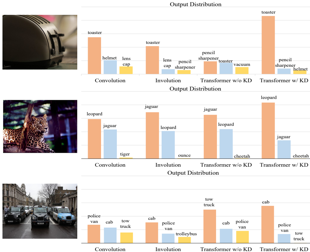
Figure 1: Class probabilities predicted by a CNN, an INN, a transformer without distillation, and a transformer distilling from both CNN and INN. CNN and INN provide come up with consistent (the first row) or complementary (the second and third rows) conclusions to correct transformer’s prediction.
