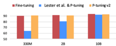
Figure 1: Average scores on RTE, BoolQ and CB of SuperGLUE dev. With 0.1% task-specific parameters, P-tuning v2 can match fine-tuning across wide scales of pre-trained models, while Lester et al. (2021) & P-tuning can make it conditionally at 10B scale.
